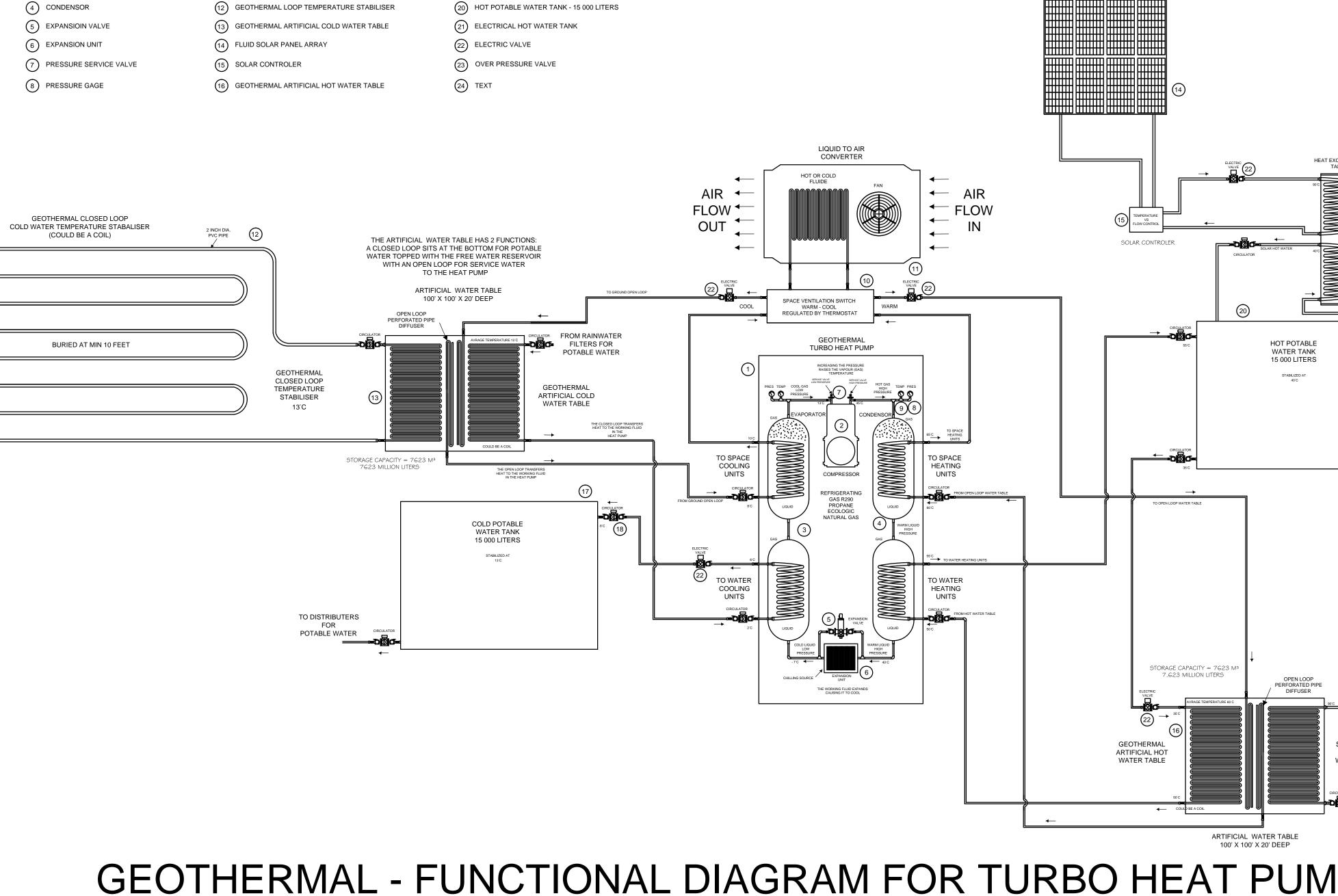
GEOTHERMAL TURBO HEAT PUMP (10) WARM - COOL - SWITCH COMTROLED BY THERMOSTAT 3 EVAPORATOR 11 LIQUID TO AIR CONVERTER
